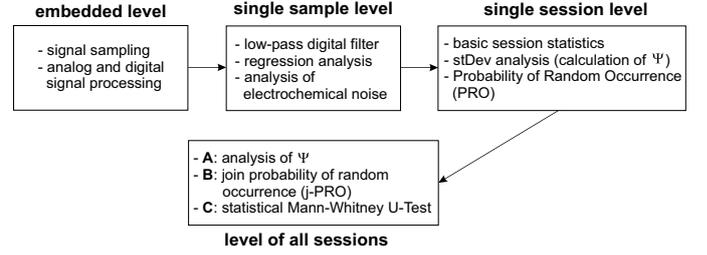
Figure 3. EIS data processing at four levels: in the device (embedded), at the levels of single samples and single sessions, as well as on the level of all sessions.
