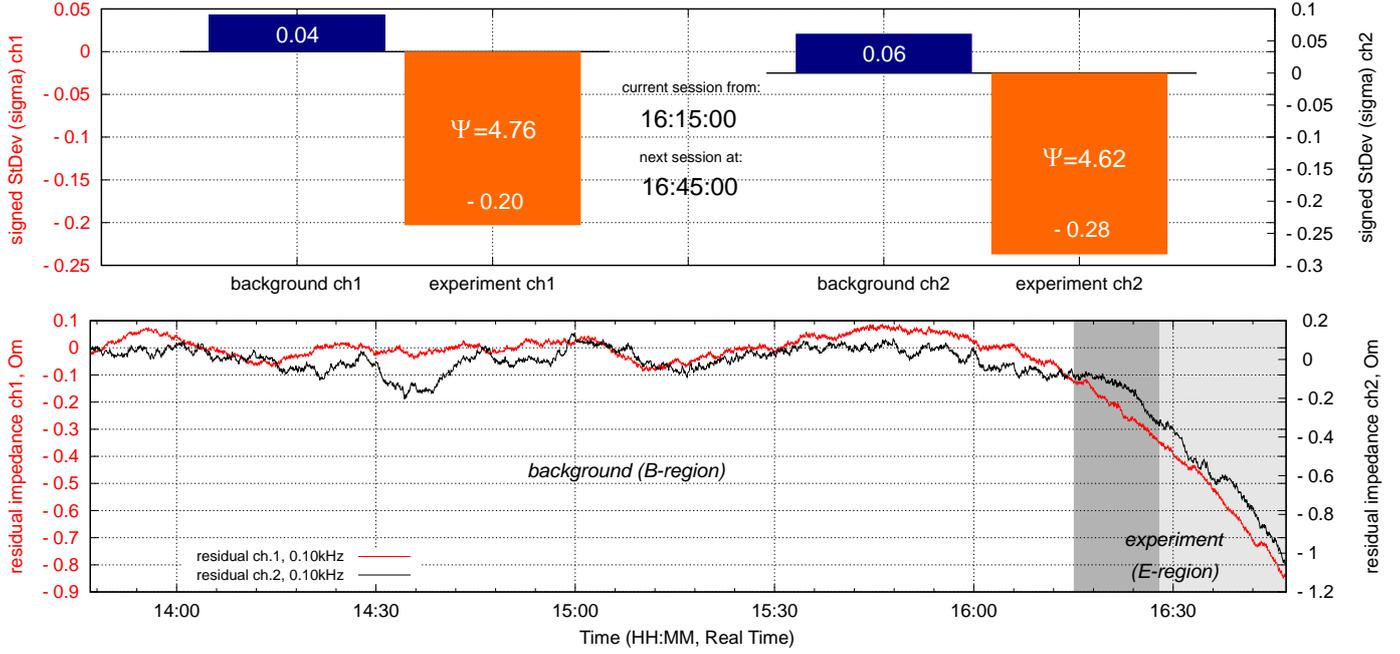
Figure 4. Example of graphical output: (upper graph) bar graphs represent standard deviations in the background and experimental regions of channels 1/2 and '3 sigma rules', the corresponding experimental graph turns orange with a significant change in  $\Psi > 3$  and 'experimental  $\Psi$ ' averaged  $\Psi$ '; (lower graph) residual dynamics of both channels after regression analysis. The gray bar indicates progress of the session.
