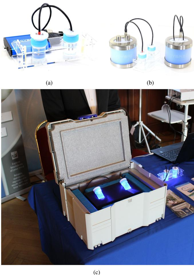
Figure 1. CYBRES EIS differential impedance spectrometer, versions with (a) open electrodes and optical excitation; (b) thermostating fluid samples; (c) a thermostabilized neopor container and thermo-compensating gel inside (exhibition 'Complementary Medicine 2019', Heidelberg, Germany), trademarked as the M.I.N.D. system.
