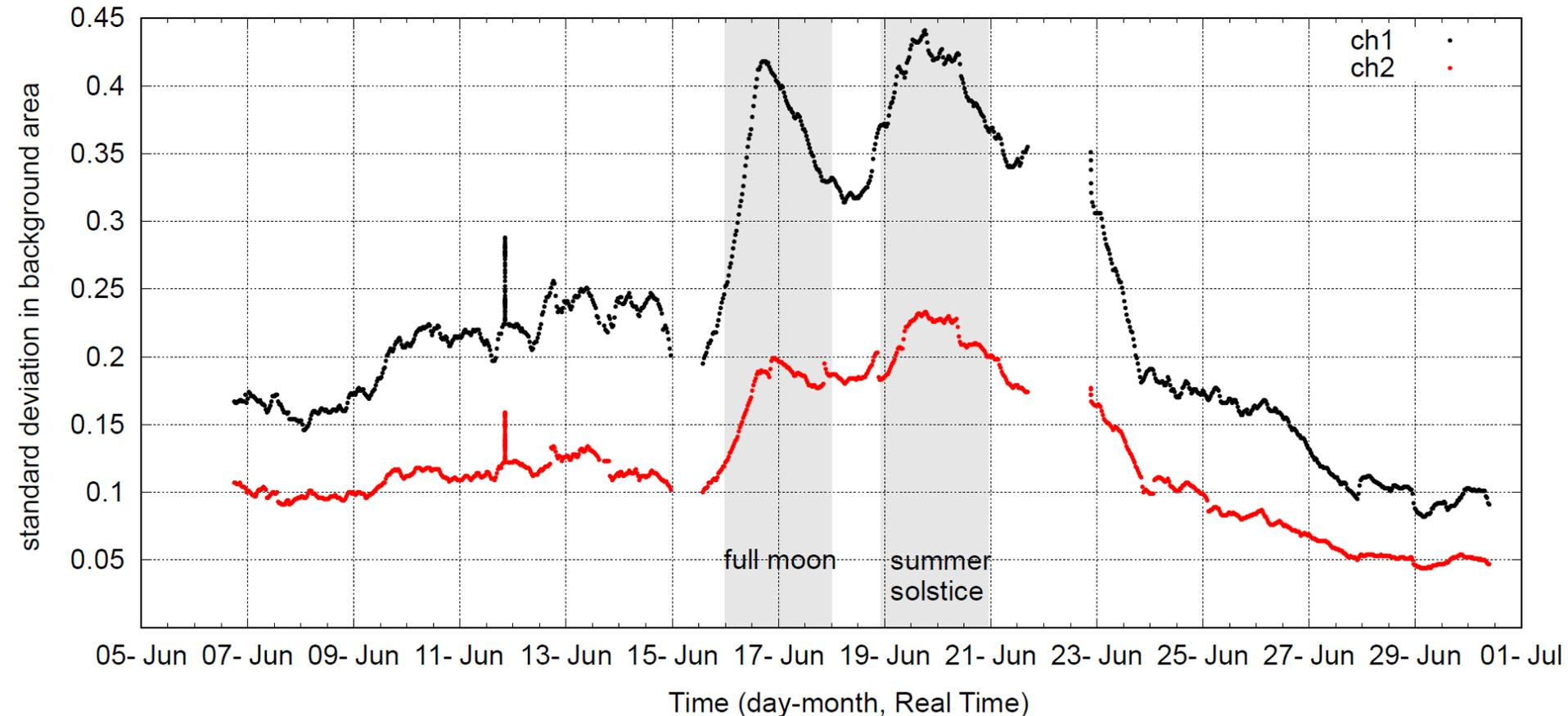
MIND sensor without public access, June 2019, shown is the standard deviation in background region, averaged in a sliding window of 24 hours. The first peak coincides with the full moon on June 17 and the second peak on June 21 – with the summer solstice.
