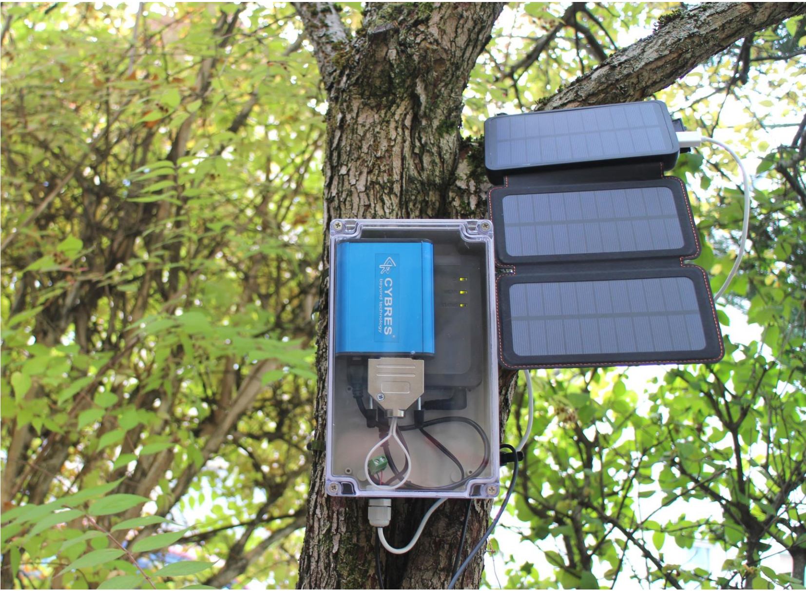
Outdoor setup, tree biopotential measurement, CYBRES, Device ID:336030
