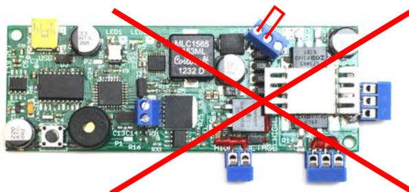
The L input should never be connected to 18/40V output when the supply voltage  $V_{EX}$  (high current) is connected to the back connector of the module - this can destroy the voltage converter.
