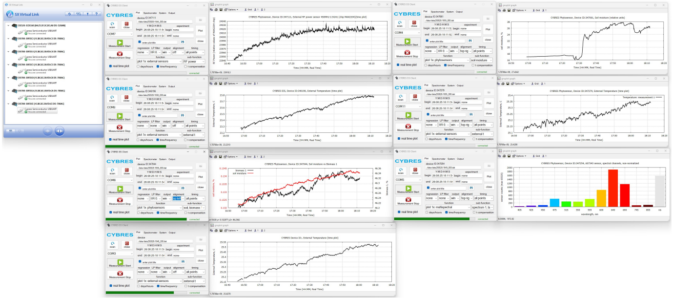
Fig. 2. Example of reliability tests: seven remote phytosensing systems connected to one PC with 'SX Virtual Link' and client software via combination of DS700AC and DS500AN modules. The system processes 644 channels (343 physical and 301 virtual) across the seven sensor systems with 1 sps sampling rate.
