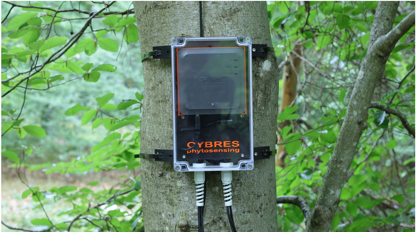
Fig. 1. Example of outdoor phytosensor system for ecological monitoring with WiFi connectivity (Silex DS500AN module).
