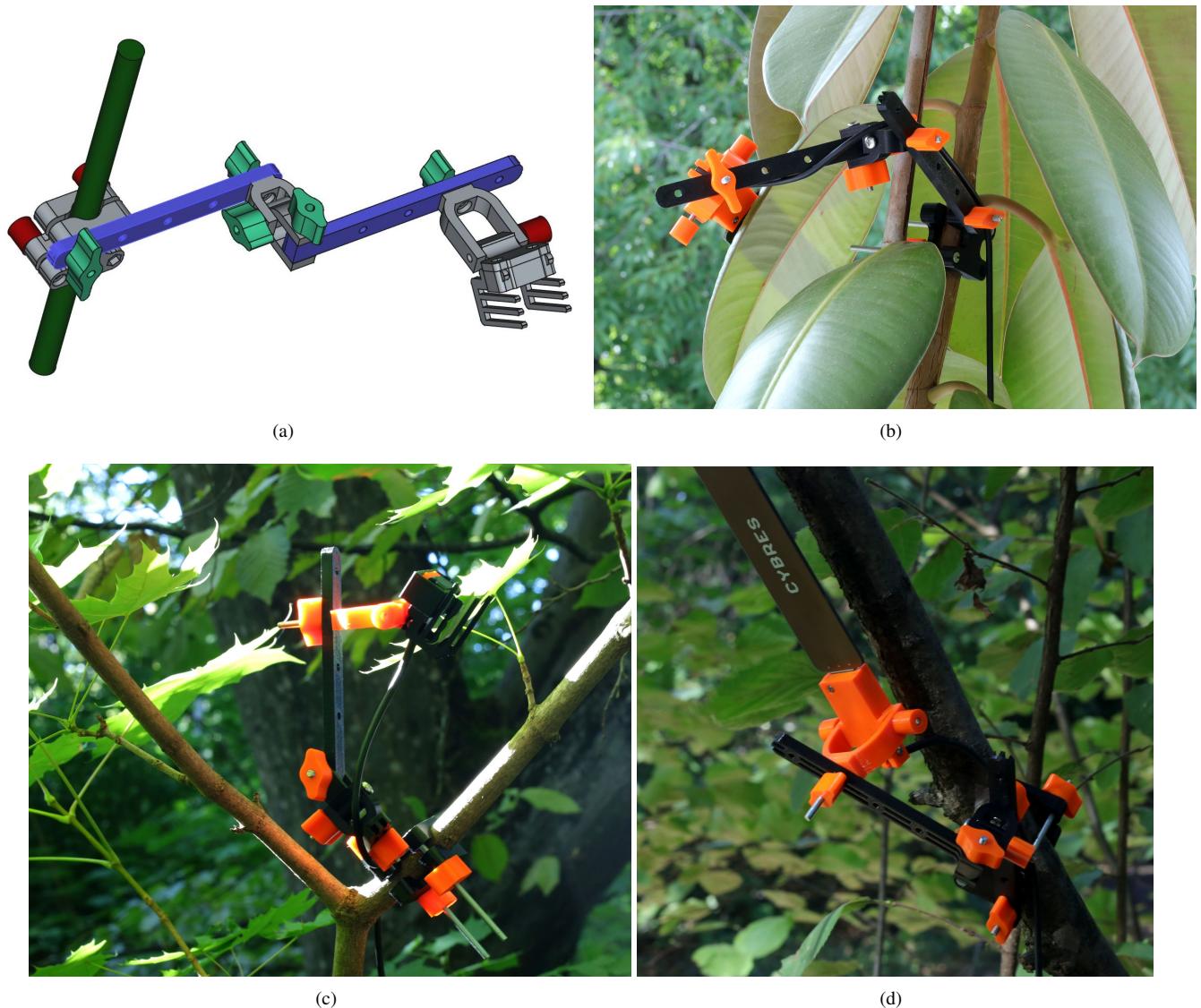
Fig. 8. 7DoF positioning arm for mounting sensors directly on the plant. (a) 3D drawing; (b-c) Different application cases.
