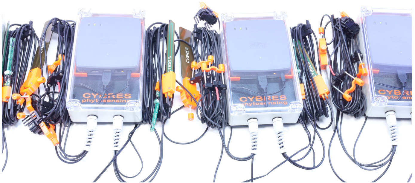
Fig. 3. Cable and sensor storage position during transportation. Removable mounting brackets can be configured with forward or backward slope.
